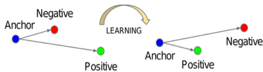
Figure 3: Triplet loss visualized [11].
