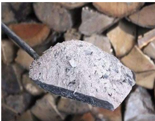
Figure 1. Wooden Waste Ash (WHA) used for experimentation
