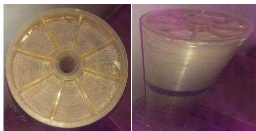
Figure 2. (a) Top view of nanofiltration membrane used for the trial, (b) Side view of nanofiltration membrane used for the trial.
