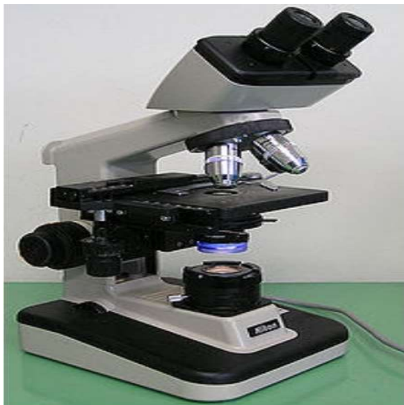
Figure 3. A Typical Optical Microscope [55]
