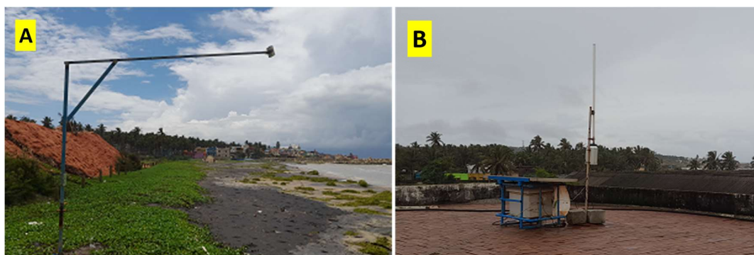
Figure 13. (A) Monitor at Valliyar river mouth, (B) Solar powered LoRa receiver
