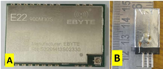
Figure 9. (A) LoRa™ module, (B) TEVISO BG 51
