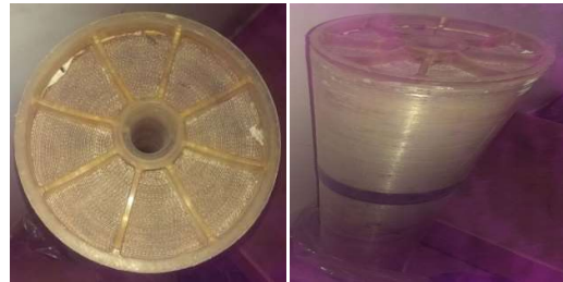
Figure 2. (a) Top view of nanofiltration membrane used for the trial. (b) Side view of nanofiltration membrane used for the trial.
