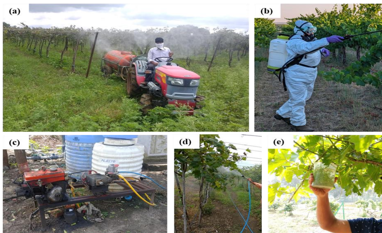
Fig. 3 Spray application technologies adopted in vineyard cultivation a) airblast sprayer, b) backpack sprayer, c, d) Horizontal triplex pump with hand spray gun, e) hand dipping
